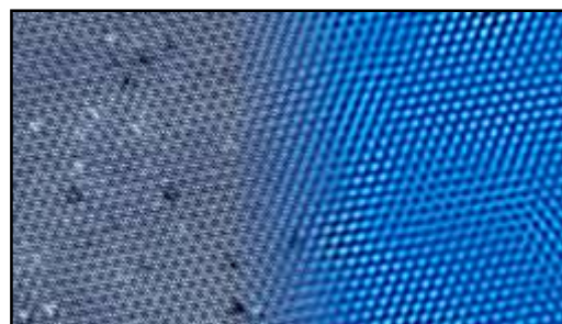
This composite image shows where the selenium atoms reside in the crystal of niobium diselenide, a transition metal dichalcogenide, using conventional scanned tunneling microscopy (left, in grey) and where the electron pairs are observed using scanned Josephson tunneling microscopy (right, in blue). Credit: Davis Lab/Provided
