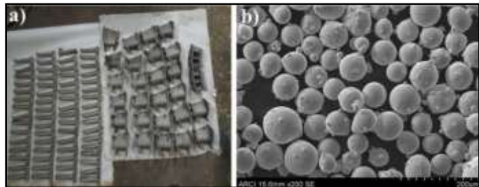
Fig 1: (a) Aero-engine components made of Ni-based superalloys for repair and (b) powder developed indigenously at ARCI
