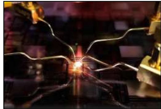
Testing routine : silicon wafers of 200 millimetre diameter with OTP memories undergo testing. | Photo Credit: Ankit Bende and Kumar Priyadarshi, IIT Bombay
