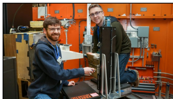
Colorado School of Mines graduate student researchers (left) Ben Schneiderman and Tim Pickle using neutrons at ORNL's High Flux Isotope Reactor to measure residual stress in welds used to make renewable energy storage tanks. Credit: ORNL/Genevieve Martin
