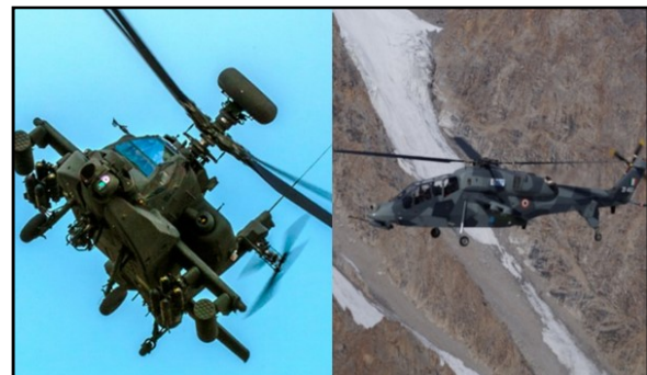
A collage of an Apache with Longbow radar atop its rotor mast (Boeing) and an LCH in Ladakh (HAL)
