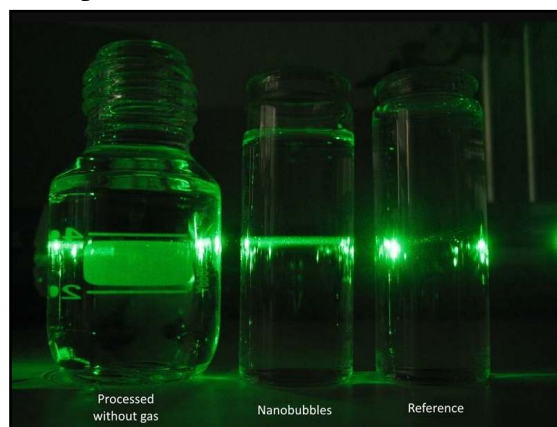
Sample in the middle scatters coherent laser light which indicates presence of nanosized bubbles. Scattering of the laser light indicates presence of surfaces. In daylight, all samples are transparent which presents that the surfaces are in nanoscale. Credit: Tapio Vehmas
