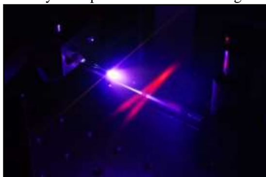
Generation of attosecond pulses in a jet of neon gas. The excitation of the gas atoms makes the intersecting infrared laser beams (in red) in the resonator visible to the human. Credit: Thorsten Naeser
