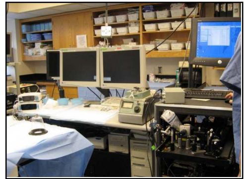
The researchers showed that ILSI can be used to identify plaques that were most likely to rupture under physiological conditions. Pictured is the animal catheterization laboratory with the portable ILSI system on the cart (right). Credit: Seemantini Nadkarni, Wellman Center for Photomedicine
