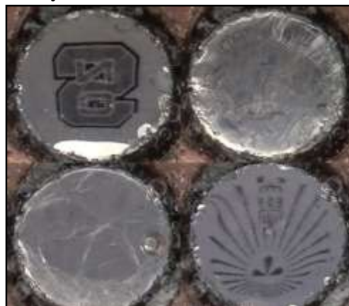
Researchers have developed a way to dynamically switch the surface of liquid metal between reflective (top left and bottom right) and scattering states (top right and bottom left). When electricity is applied, a reversible chemical reaction oxidizes the liquid metal, creating scratches that make the metal scattering. Credit: Keisuke Nakakubo, Kyushu University
