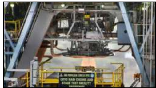
The qualification test of the cryogenic engine of the human-rated GSLV rocket for Gaganyaan programme going on at ISRO Propulsion Complex (IPRC), Mahendragiri, Tamil Nadu on Wednesday.
