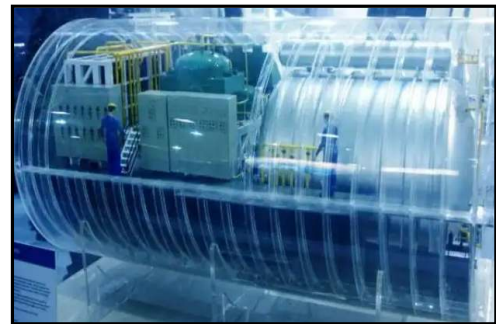
Indian Fuel Cell Based Air Independent Propulsion (AIP) System
