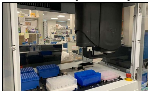
GIFS' liquid handling robot used to automate the dispensing of specific amounts of liquids to containers in the lab. Credit: Pierre-Luc Pradier.
