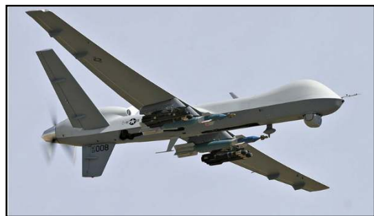
A US Air Force MQ-9 Reaper armed with bombs and air-to-ground missiles | General Atomics
