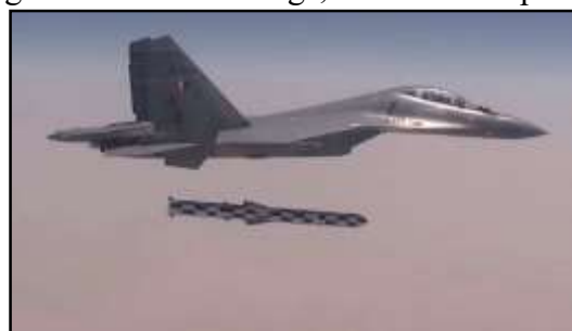
The BrahMos missile being launched from IAF's Sukhoi-30 MKI in the Bay of Bengal. (Via Twitter)
