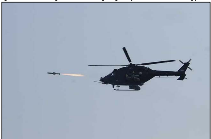
HELINA anti-tank missiles were launched from ALH Dhruv helicopter for evaluating missile capabilities in minimum and maximum range of 7 kms
