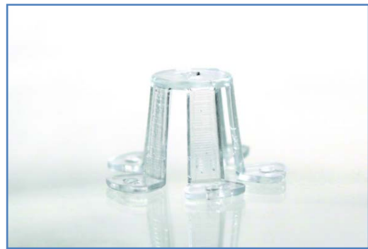
Complex structures of transparent fused silica fabricated via injection molding of the newly developed Glassomer composite. Credit: Glassomer GmbH
