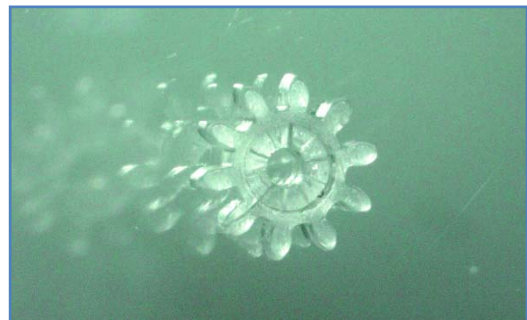
Transparent fused silica gears produced by injection molding of the newly developed Glassomer composite. Credit: Glassomer GmbH
