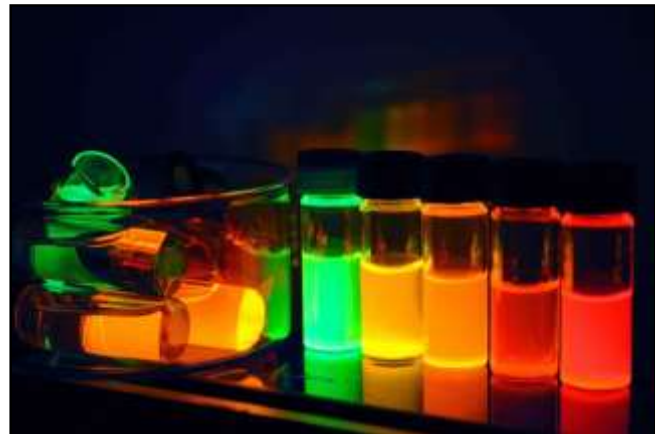
The tiny specs of matter called quantum dots can be tuned to emit light in specific wavelengths. That's just one quality that makes them valuable in a range of technology applications. Credit: Los Alamos National Laboratory
