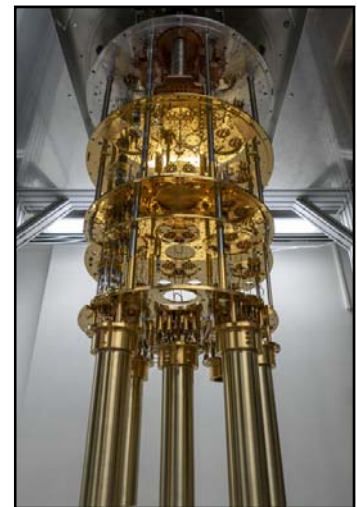
The dilution fridge at UCL. Credit: A. Abrusci / UCL
