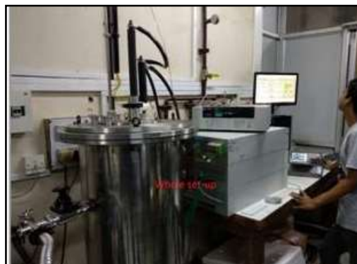
The figure above shows the fully integrated smart superconducting fault current limiter in operation.
