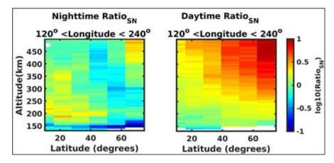
The hemispheric asymmetry in terms of variation of Ratio of southern hemisphere (SH) to northern hemispheric (NH) electron density (ne) as a function of latitude and altitude. It represents the ratio of ne in a SH latitude to that in a NH latitude. The left and right panels represent night- and dayside conditions. The color codes shows the ratio in log10 scale, in each 5 km altitude by 10° latitude bin. The white spaces represent data gap.
