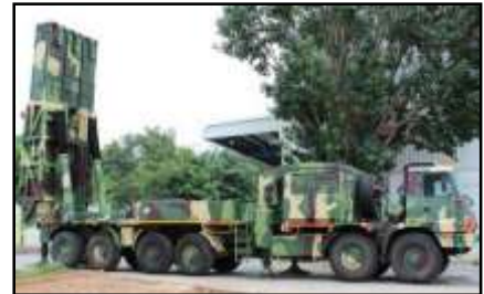
TEL Transporter Erector Launcher vehicle of Indian Advanced Air Defense anti-ballistic missile system. (Picture source Twitter account Defense Decode®)
