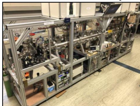
The 4.5-meter long experimental setup. On the left, the chamber in which the strontium fluoride molecules are created. Credit: Steven Hoekstra, University of Groningen
