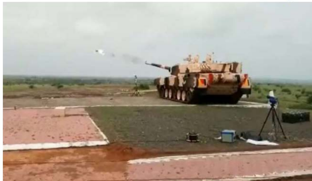
Engaging the targets at lower ranges is a challenge due to the dimensional constraints of tank launched ATGMs, which has been successfully accomplished by the ATGM for MBT Arjun.
