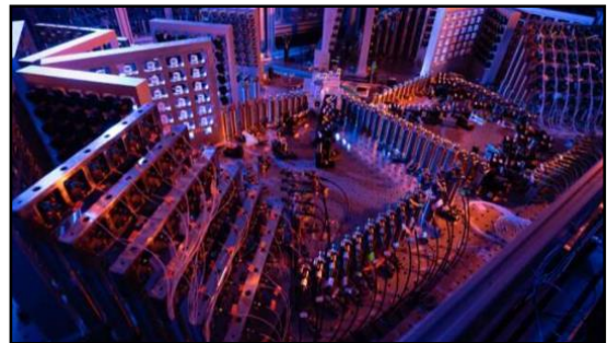
The Pan team's optical quantum computer uses a 144-mode interferometer to solve a Gaussian boson sampling problem with a factor-of-1024 speedup in computational time relative to a classical computer. Credit: Chao-Yang Lu/University of Science and Technology of China, via Physics
