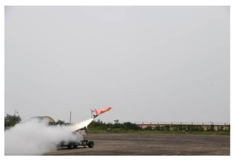
The trials were carried out with improved Radar Cross Section, Visual and Infrared augmentation systems. During the trials, various mission objectives covering safe release of booster, launcher clearance, and endurance performance were successfully validated. Two launches were conducted back-to-back within a gap of 30 minutes, demonstrating the ease of operation with minimum logistics. Representatives from the Services witnessed the flight trials.
