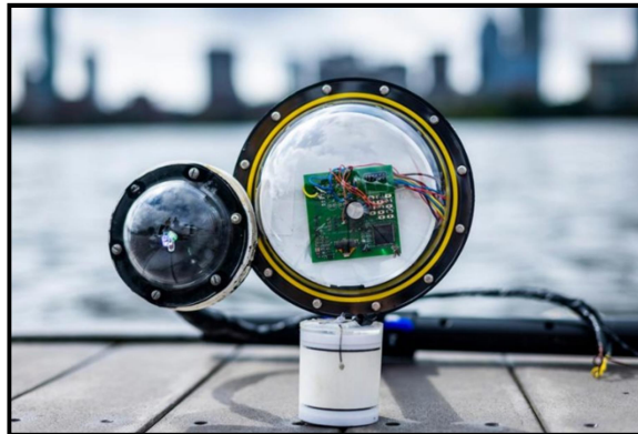
A battery-free, wireless underwater camera developed at MIT could have many uses, including climate modeling.
