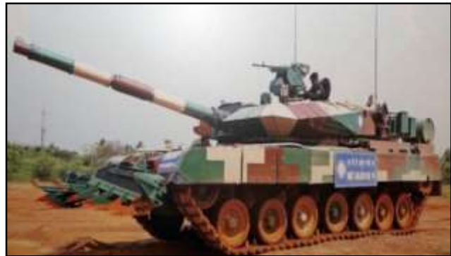
The MBT Mk-1A is a new variant of Arjun Tank designed to enhance fire power, mobility and survivability, infused with 72 new features and more indigenous content from the Mk-1 variant. Image Courtesy: @DRDO_India/Twitter
