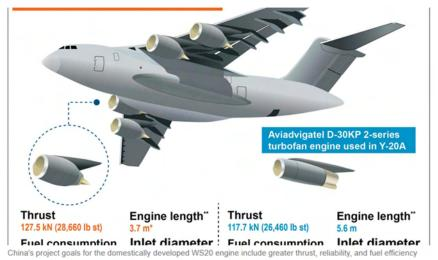
compared with Russian engines currently powering the XAC Y-20A transport aircraft. (Janes)
