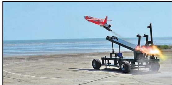
Abhyas aerial vehicle being test flown from ITR
