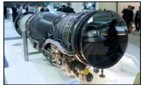
M88-4E afterburning turbofan engine for Dassault Rafale (Wikimedia Commons)
