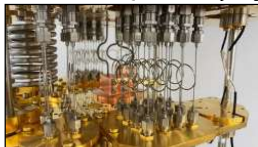
A dilution refrigerator that houses qubits. Credit: RIKEN Center for Quantum Computing
