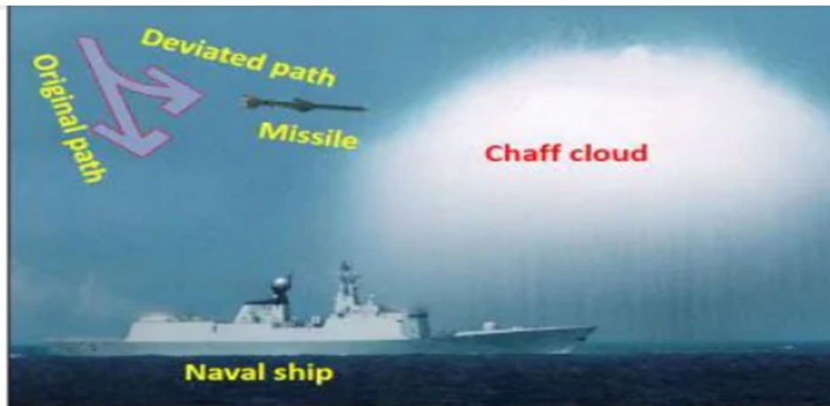
CHAFF creates a metal particle cloud near the warship and deflects the missiles from it.
