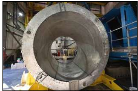
On October 7, 2021, crews at Brookhaven National Laboratory installed the 1.4-Tesla, 20-ton superconducting solenoid, which will be the centerpiece of the sPHENIX upgrade. Credit: Brookhaven National Laboratory
