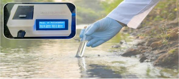
Once interfaced with an in-house, multi-channel monitoring apparatus, the MopR-based sensor forms the core of the newly developed aromatics tracking device—AroTrack. Talking about how the AroTrack detects the pollutants using the biosensor modules, Prof. Bandyopadhyaya explains, "AroTrack contains a light emitting diode (LED)-phototransistor assembly, that shines a light of
