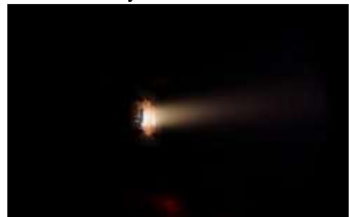
Side view of a flight model of the NPT30-I2 iodine electric propulsion system firing in a vacuum chamber. Credit: ThrustMe
