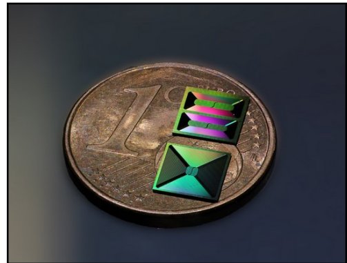
Integrated silicon nitride photonic chips with meter-long spiral waveguides. Credit: Jijun He, Junqiu Liu (EPFL)
