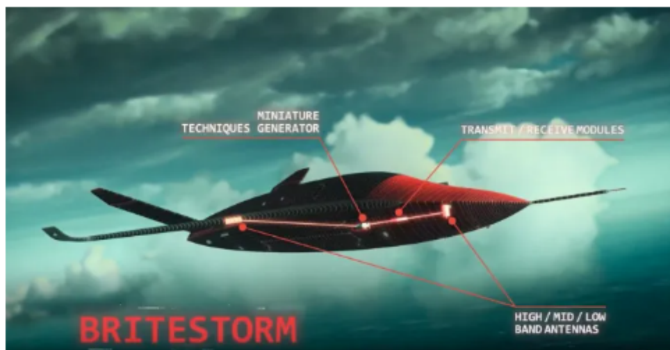
Diagram showing the components of a BriteStorm payload – the Miniature Techniques Generator (MTG), Transmit Receive Modules (TRMs), and high/medium/low band antennas.
