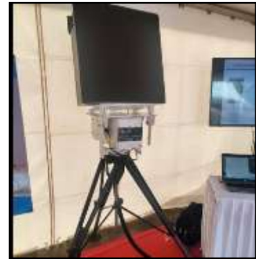
The radar can be controlled and operated remotely through wired communication, it is portable and easy to deploy.
