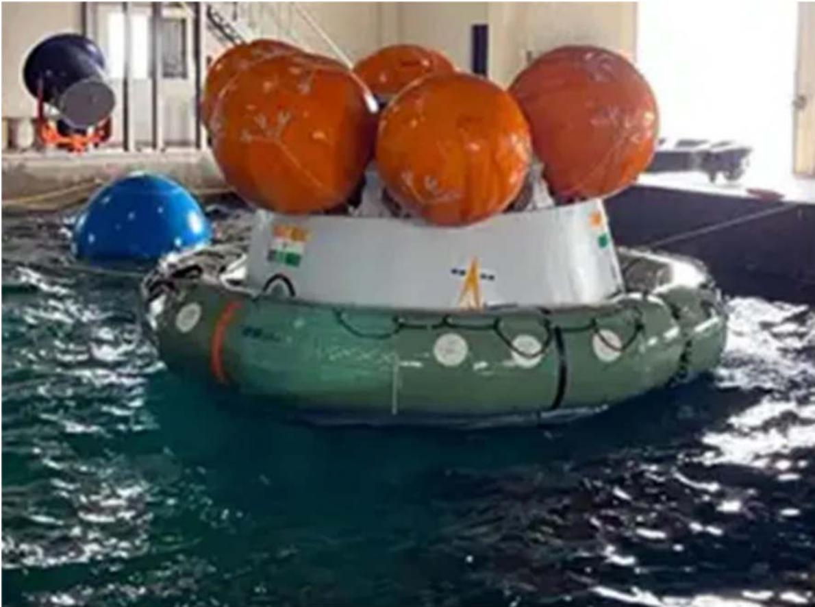
The orange floats are used to keep the capsule oriented the right way in choppy seas. (Image credit: ISRO).
