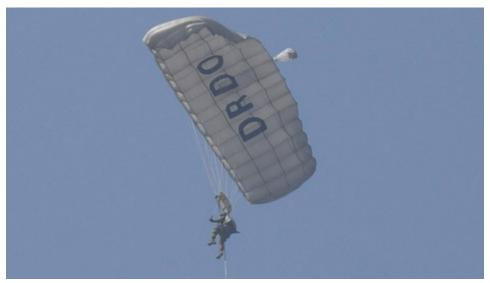
MCPS is a sophisticated parachute system designed for military operations, particularly for special forces. It allows paratroopers to jump from aircraft with a combat load, deploy their parachutes at predetermined altitudes, and navigate and land safely.
