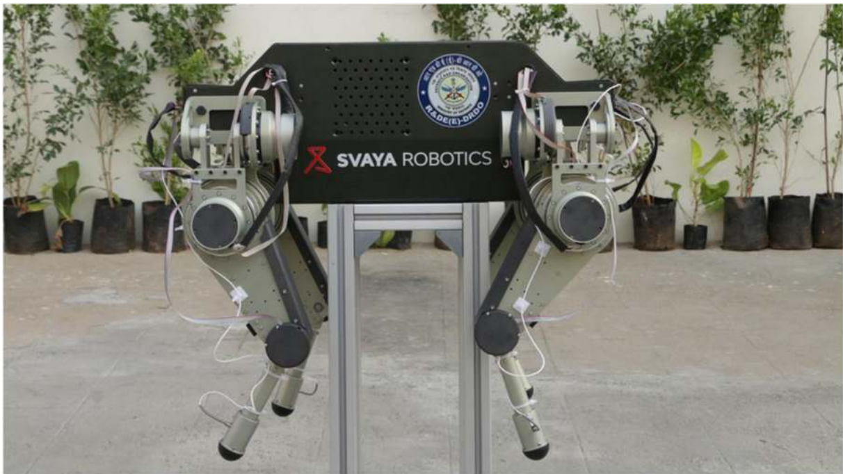
The quadruped robot is for navigating in unstructured terrains to provide remote reconnaissance and inspection for the defence and security forces. | Photo Credit: Arrangement
