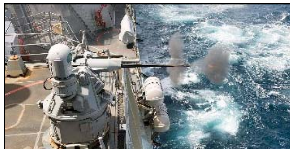
A MK 38 Mod 2 gun on a US Navy ship; the gun is a variant of the Israeli Typhoon RWS | Via Wikimedia Commons
