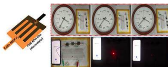
Figure 3. Graphical representation of the planar device and demonstration of the planar device's practicality via the operation of the clock watch and LED illumination.
