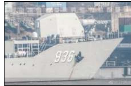
China's Type 072III-class landing ship Haiyang Shan is outfitted with a large weapon that has been identified by some analysts as a railgun. (via Twitter)
