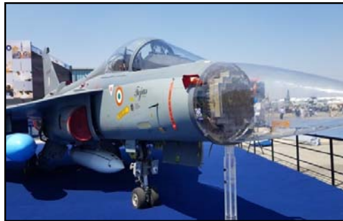
Active Electronically Scanned Array (AESA) radar (via DRDO)
