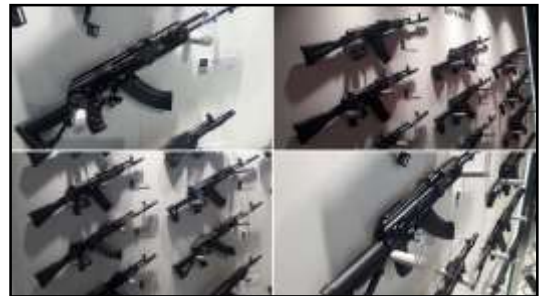
AK-203 Assault rifle is of 7.62mm calibre, with 39 calibre length barrel, i: e to say that the length of its barrel is 39 times the calibre – 7.62 X 39 mm.
