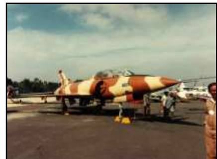
The Marut was capable of carrying 1,800 kg of bombs, 100 rockets (68 mm) and four 30 mm cannons.(Photo caption: Wikimedia commons)
