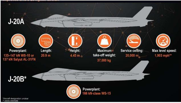
A new variant of the CAC J-20 fifth-generation fighter includes design changes to improve low-observable characteristics and aerodynamics. This variant appears to have also been equipped with the new WS-15 powerplant. (Janes)
