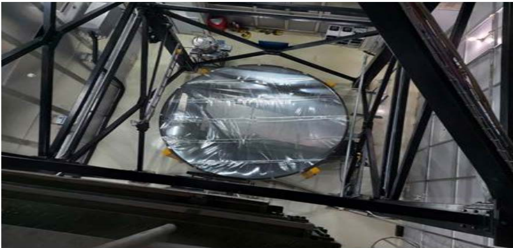
Top view of the ILMT located at the Devasthal Observatory of ARIES showing the liquid mercury mirror covered by a thin mylar film.
