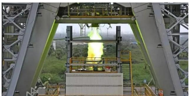
During the three-second test, the engine was ignited and operated at up to 60% of its rated power, performing with stability and control throughout. The PHTA, which includes all major components of the engine except the thrust chamber, is designed to evaluate the propellant feed system, including low- and high-pressure turbo pumps, pre-burner, start systems, and control mechanisms.
