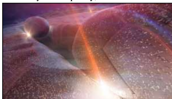
Artistic view of the nanoparticle-in-groove plasmonic cavities. Molecules cover the gold film and are sandwiched between the groove and the 150-nm large nanoparticle. The infrared signal of interest comes from below the substrate while the pump laser providing energy for upconversion comes from the top. Both are focused by the cavity onto the molecules, and interact with their internal vibrations to generate an upconverted copy of the infrared signal at visible frequencies (bright spot). Credit: Nicolas Antille
